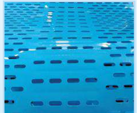
Elliptical perforations for preventing product loss
