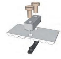
TAS150 - suitable for AT10 profile, 50 mm wide, two pins at 25 mm centre distance
