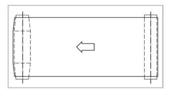
With conveyor aspect ratio (conveyor length to belt width) in excess of about 5 to 1 and in installations with reversing operations, it is advisable to crown both, head pulley and tail pulley.
