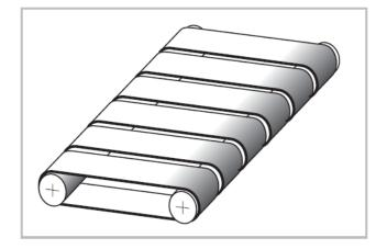
In cases where the application does not require a wide belt, the use of several narrow belts is recommended. The tracking can be controlled much easier.
