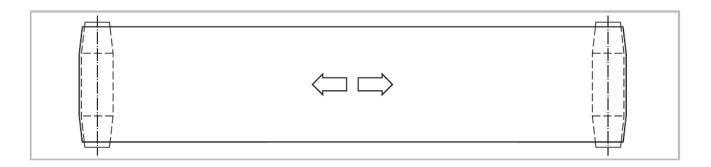
Following this method, a correctly aligned belt can be maintained in its central position as long as there is no excessive deflection of the pulleys.
