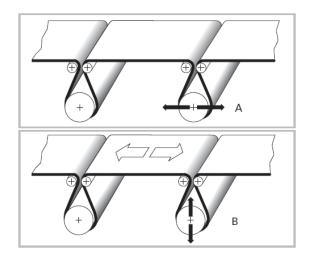
In areas where local transverse forces occur, tracked belts will be kept in place by additional belt wraps. The effect can be enhanced by covering the additional pulleys.
