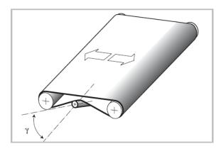
Advisable for guiding wide belts with short conveying distances are inclined rollers on the return side.
