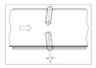
Cylindrical rollers are installed at the belt edges and angled forward in the belt running direction. The skew angle,  $\gamma$ , should be 3° to 12° depending upon belt load, the friction between roller and belt, and on the belt speed.
