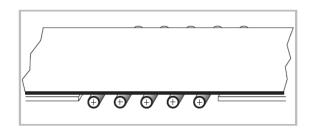
Local transverse forces can also be dealt with by installing multiple carrying rollers with friction cover. This method is suitable both for installations with slider bed and carrying rollers. With rollers adjusted exactly perpendicular to the belt running direction, the tracking will also work for reversing operation.
