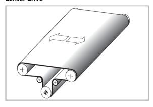
Center drive is recommended for reversing operation. The driving pulley should be cylindrical-conical and, if required, lagged. Head and tail pulley as well as deflection rollers are of cylindrical shape.
