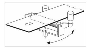
This tracking device is used for heavy belts and for belts with high lateral stability. Specialty manufacturers supply these units, which can also be equipped with adjustable sensors that substantially reduce belt edge wear.
