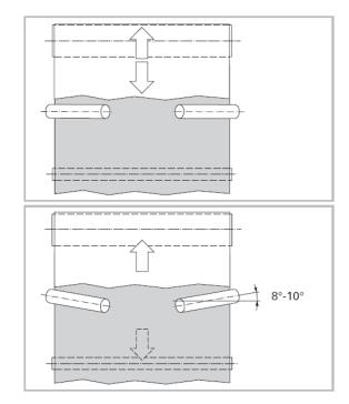
Inclined rollers on the return side have also proven successful for tracking wide, short belts and with thin belts at high speeds. In this case driving pulleys and tail pulleys are to be fitted with cylindrical profiles in order to avoid folding or creasing.
