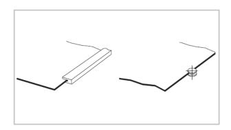
This tracking measure is only possible for belts with sufficient lateral rigidity and edge integrity, however, belt edge wear will increase. Guide rollers are preferable to lateral wear strips in this respect.
