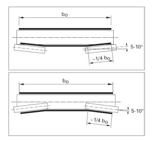
To achieve a satisfactory tracking effect, the belt contact of a roller should be around ¼ of the belt width and the rollers angle of incline should be 5° to 10°.
