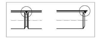
Short, wide belts can be guided effectively by using guiding profiles, provided there is sufficient belt transverse rigidity and fairly low speed. It is advisable to guide the belt in the pulleys rather than in the slider bed. This means, the grooves in the pulleys should be narrower than those in the slider bed.
