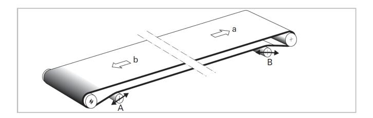
Guiding pulley A tracks the belt correctly in running direction a, guiding pulley B tracks the belt correctly in running direction b.
