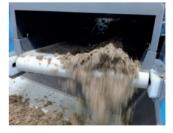
**Abrasion resistant** Suitable for abrasive products, or where scrapers or side skirts are used.
