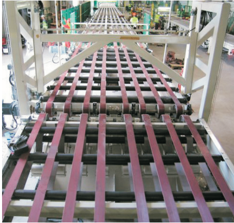
ASTER 24QF at the transfer line to the oven.
