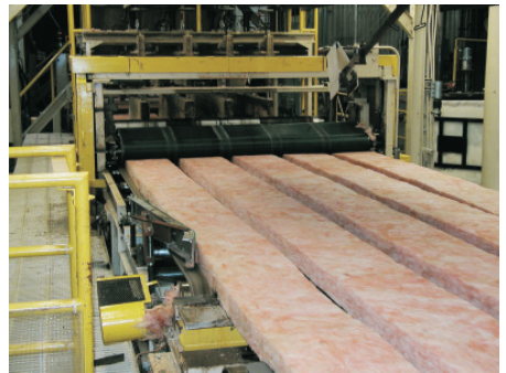
BREDA 25CF inclined conveyor to the oven.
