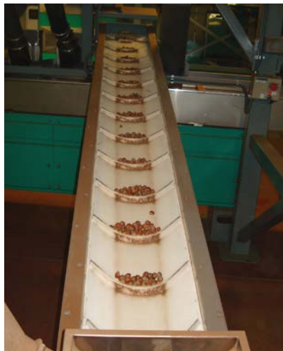
Troughed conveyance of filberts.
