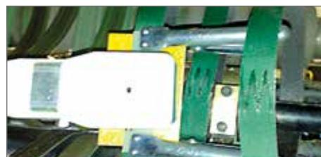
With the Chiorino **FAST JOINT KIT** the **PT®** machine tapes can be made endless on site in a few minutes, reducing the maintenance time.
