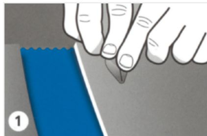
Score the back and lubricate the pin.
