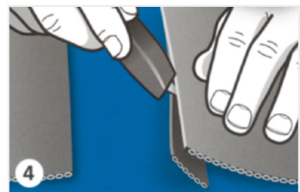
Carefully cut the top cover.
