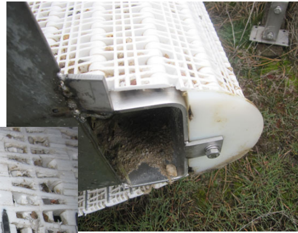
Dirt, soil and stones that have to be separated from the product get stuck in the holes in modular belts.
