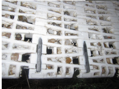
Dirt, soil and stones that have to be separated from the product get stuck in the holes in modular belts.
